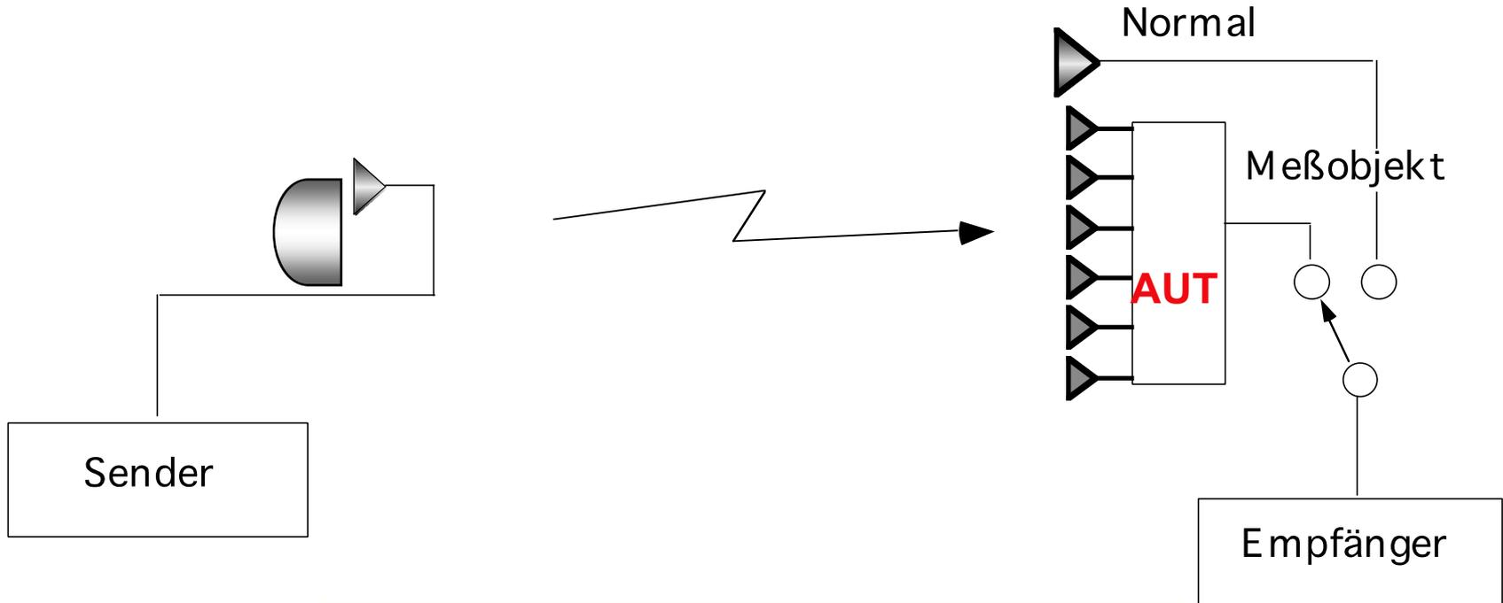
$$G_{AUT}|_{dB} = G_{Normal}|_{dB} + 10 \log \frac{P_{E \text{ Messobjekt}}}{P_{E \text{ Normal}}}$$
